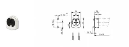
L1+19: Recommended dimension - The distance between the cut-outs and the tolerance should be governed by the dimensions of the respective lamps and luminaires.
