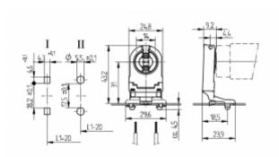
L1-20: Recommended dimension - The distance between the cut-outs and the tolerance should be governed by the dimensions of the respective lamps and luminaires.
