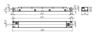
• Casing: M10 Ref. No.: 186696 • Length: 359 mm • Width: 30 mm Height: 21 mm
